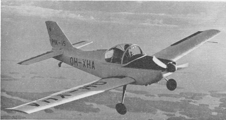
Designed and built by the Polyteknikkojen Ilmailukerho, Helsinki, Finland, the PIK-15 is a side-by-side two-seater of wooden construction, powered by a 150-h.p. Lycoming and intended primarily for glider towing. First flight was on 29th August
