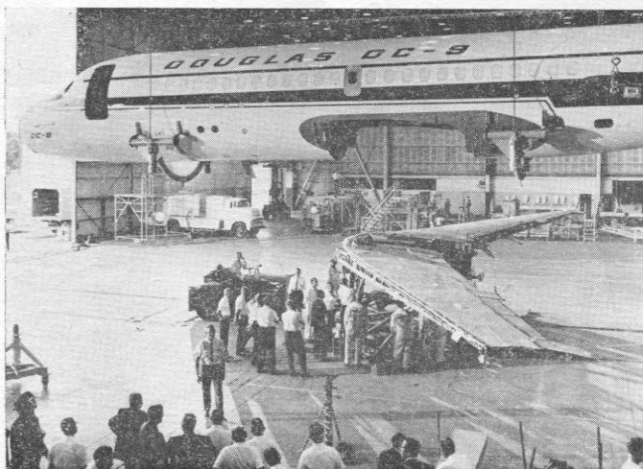
A milestone in the development of the Douglas DC-9 was reached on 20th October when the fuselage of the first prototype was mated to its wings. The machine will be ready for roll-out in January and is expected to fly in March
