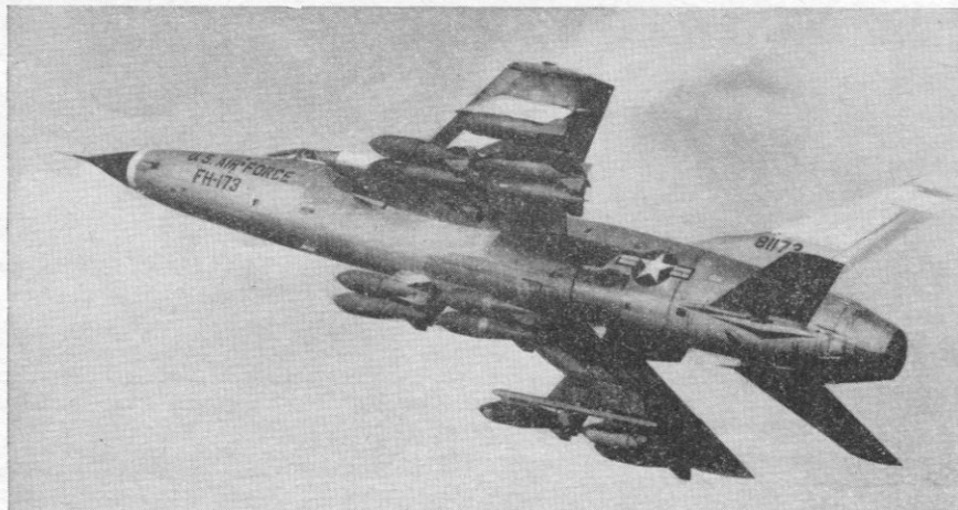
LEFT: F-104C Starfighters of the 479th TFW, George AFB, California. The only tactical fighter wing flying this type, the 479th is to convert to F-4C Phantoms this winter. ABOVE: The Thunderchief, which equips seven wings, can carry up to 13,000 lb. in external stores (F-105D illustrated with 16 x 750-lb. bombs). BELOW: The F-4C Phantom, already serving with two wings, is scheduled to equip five more
