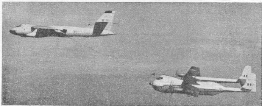
Believed to be the first photograph showing an Argosy C.1 being refuelled in flight, from Valiant XD812—taken during trials at Boscombe Down
