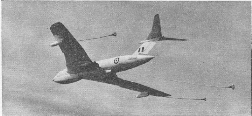
The first Victor tanker (XA918) displays its three-point flight refuelling equipment, capable of handling anything from Lightnings to turboprop transports
