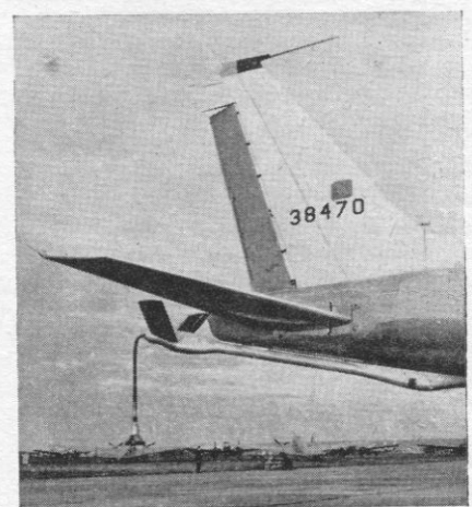
ABOVE: A Mirage IVA refuels from a Boeing KC-135F. Twelve KC-135Fs have been supplied to the French Air Force; when not engaged in flight-refuelling duties, they will be available for normal transport work. RIGHT: A close-up of the Boeing "flying-boom gear", which was developed from the British Flight-Refuelling Ltd. system
