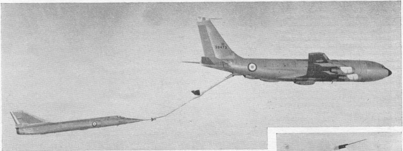
ABOVE: A Mirage IVA refuels from a Boeing KC-135F. Twelve KC-135Fs have been supplied to the French Air Force; when not engaged in flight-refuelling duties, they will be available for normal transport work. RIGHT: A close-up of the Boeing "flying-boom gear", which was developed from the British Flight-Refuelling Ltd. system
