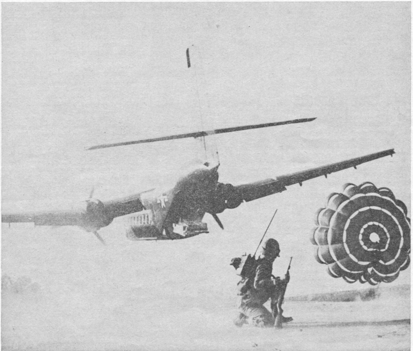
This is an actual photograph of CV-2B CARIBOU performing a Low Level Extraction (LOLEX) drop.
