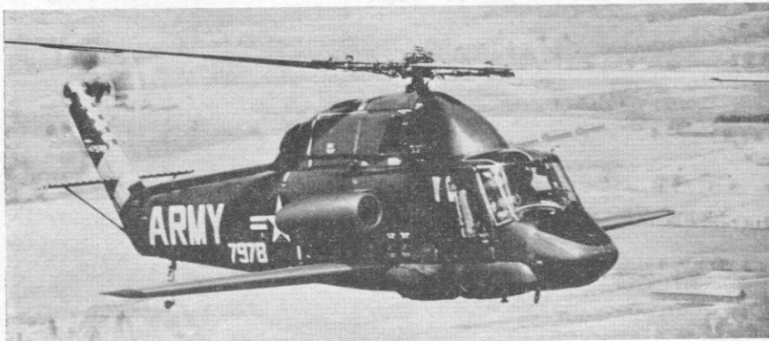
BELOW: Fitted with wings, and with jet-thrust augmentation, the Kaman UH-2 will be used for research at speeds of over 250 m.p.h.
