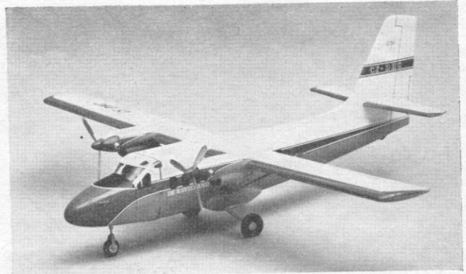
D.H. Canada have started production of a new short-field, short-haul utility aircraft, the Twin Otter, shown here in model form. Powered by two 550-s.h.p. Canadian P. & W. PT6As, it will carry up to fourteen passengers over 100- to 600-mile stages at 160 knots
