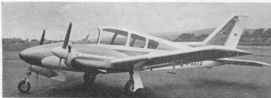
BELOW: First flown on 27th August, the Beagle 242 (G-ASTX) is a revised version of the 218 using metal instead of plastics construction
