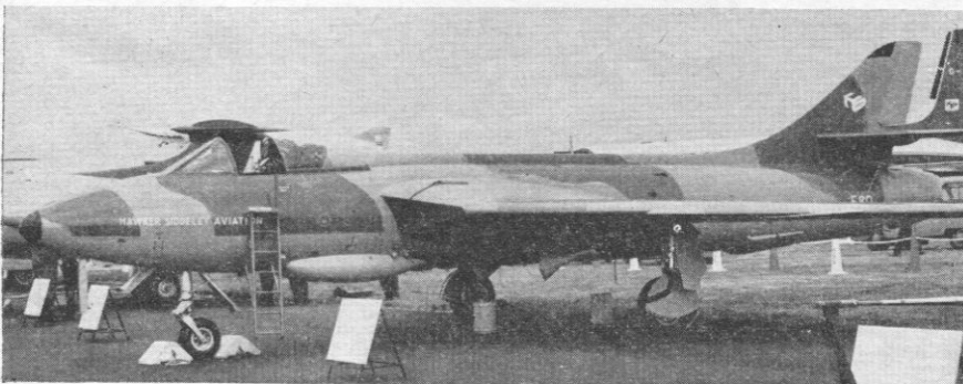
ABOVE: Hawker Siddeley Hunter "580", in desert camouflage but devoid of national insignia, believed to be an F.6 converted to Mk. 9 standard
