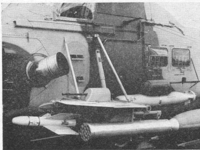
LEFT: Weapons of the Wessex HC.5 include .303 machine guns, Nord SS.11 missiles, 2-in. rockets, and homing torpedoes. RIGHT: Vulcan B.2 XM595 from Scampton bears the badges of its station and Nos. 27, 83 and 617 Squadrons
