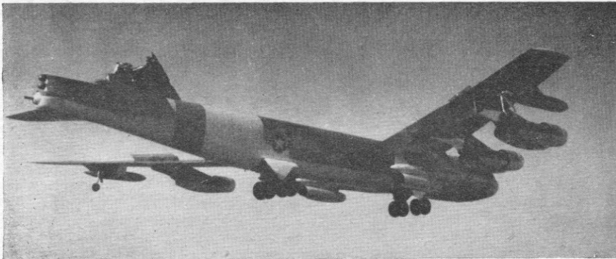
Proving that the "youngsters" can take it as well as W.W.II Fortresses, this Boeing B-52H flew for five hours and made a successful landing, on 10th January, after losing most of its 40-ft. fin and rudder. The aircraft was carrying out a "low-level test mission" at the time
