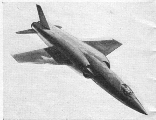
An impression of the VJ-101D, with five RB.162 lift engines (all in the forward fuselage) and two deflected-thrust RB.153s
