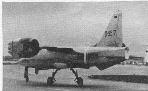
ABOVE: Three views of the EWR-Süd VJ-101C-X1, powered by six Rolls-Royce RB.145s. For vertical flight the front part of each pod moves forward leaving a gap (LEFT) to admit air for the engines, but this is closed in level flight (TOP), air then entering through the nose intakes
