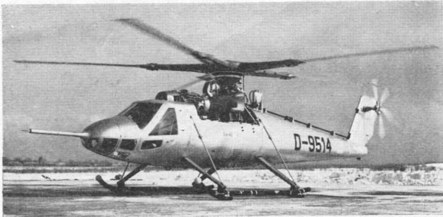
Flown in January D-9514 is the first of three Bolkow Bo 46s being built to test the Derschmidt "lead-lag" rotor system, designed to keep tip speeds within efficient limits during fast forward flight
