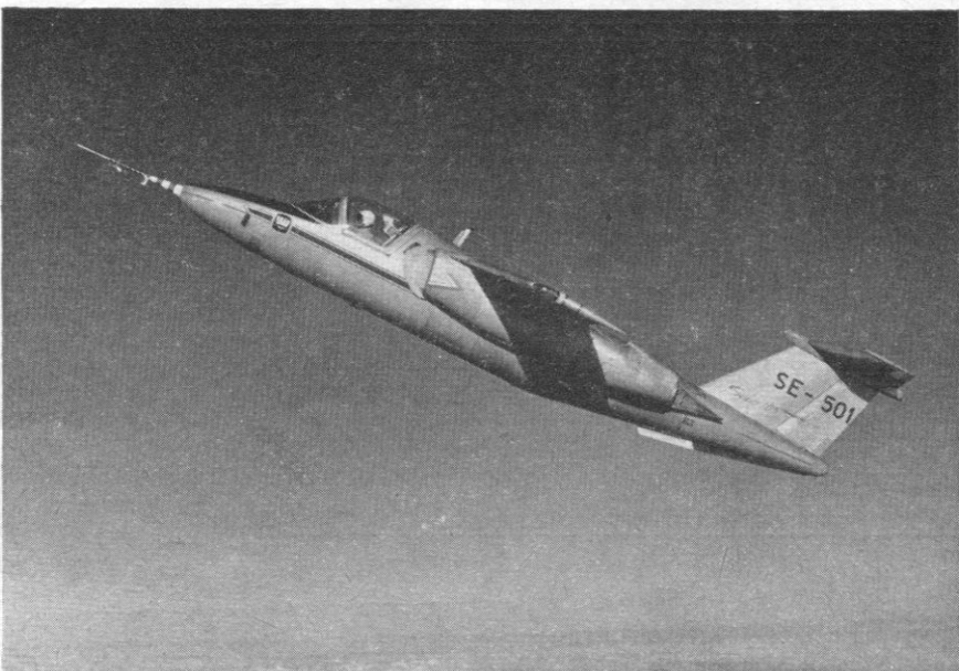
BELOW: A recent shot of the prototype Saab-105. The Swedish A.F. has ordered 130 with more powerful (1,650-lb. s.t.) Turboméca Aubisque engines
