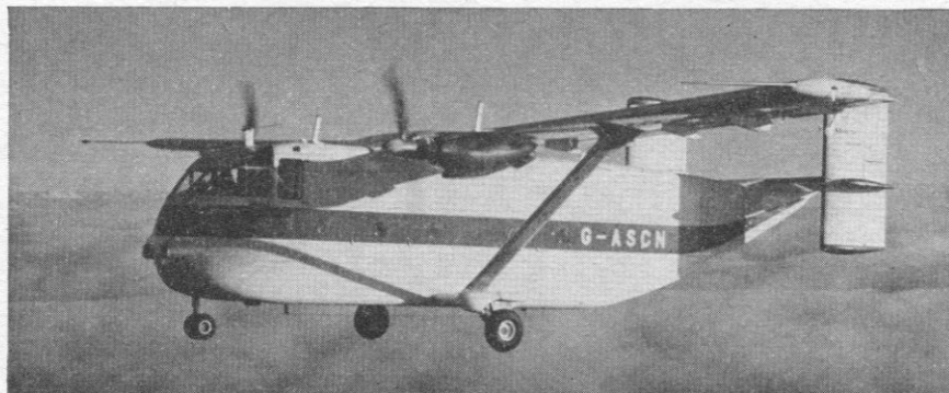
The production Turbo-Skyvan (drawing) will have a more pointed nose and lower tail than the prototype (RIGHT)
