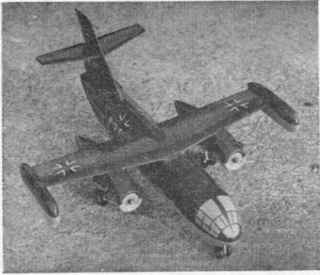
Subject of a joint Anglo-German feasibility study is the Dornier Do 31 V/STOL transport. LEFT: Model of prototype with two Bristol Siddeley Pegasus vectored-thrust engines and six Rolls-Royce RB.162s for lift; production version will be larger and with ten lift engines. RIGHT: Control problems are being investigated with this hovering rig
