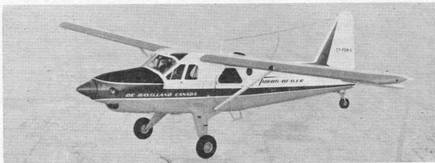
First flown 30/12/63, the prototype D.H. Canada Turbo-Beaver (578-s.h.p. Pratt & Whitney PT-6A) is the 1,525th Beaver built
