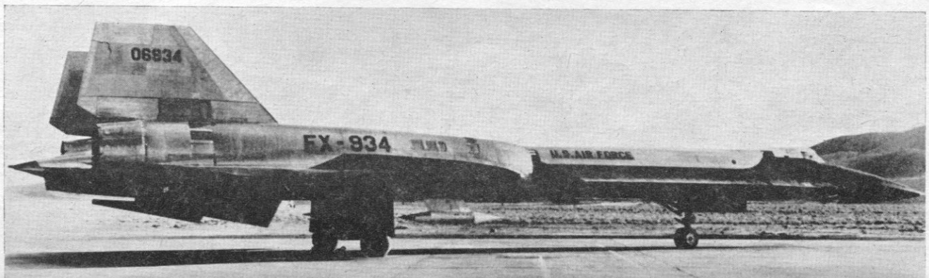
First photos to be released of the 2,000-m.p.h. Lockheed A-11 (alias "Johnson Special"?), together with provisional drawing opposite. Picture below shows central ventral fin folded for ground clearance
