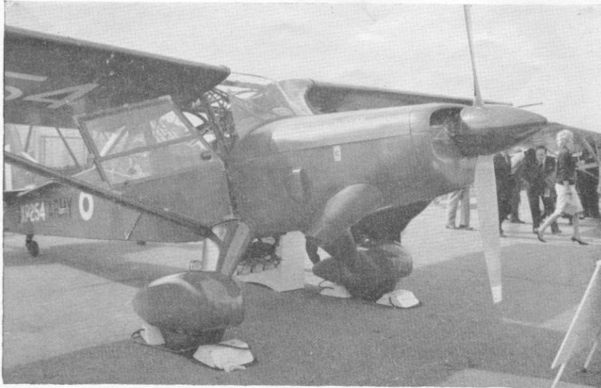
The Beagle-Auster Mk. XI with Rolls-Royce Continental engine.
