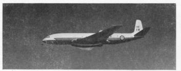
Will you fly Comets? This Comet 2 has a stage length of more than 2,200 miles against a 50 m.p.h. headwind. The cruising speed is 480 m.p.h. and the cruising altitude is 35-40,000 ft. The Comets provide the R.A.F. with that essential quality of mobility so vital in air strategy today.
