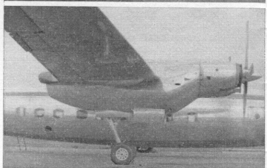
Top to bottom are close-up photographs of the Auster J-1N Alpha's Micronair spray units; the new tailplane and fins on the Saro P.531; the starboard Rolls-Royce Tyne turboprop engine of the Airspeed Ambassador test-bed. (Air Pictorial photographs.)
